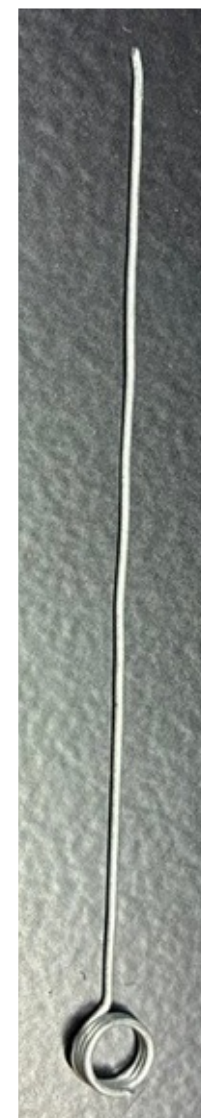
Needle-pointer, fashioned from straightened steel wire.
