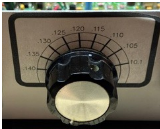
Dial, missing its needle-pointer.
