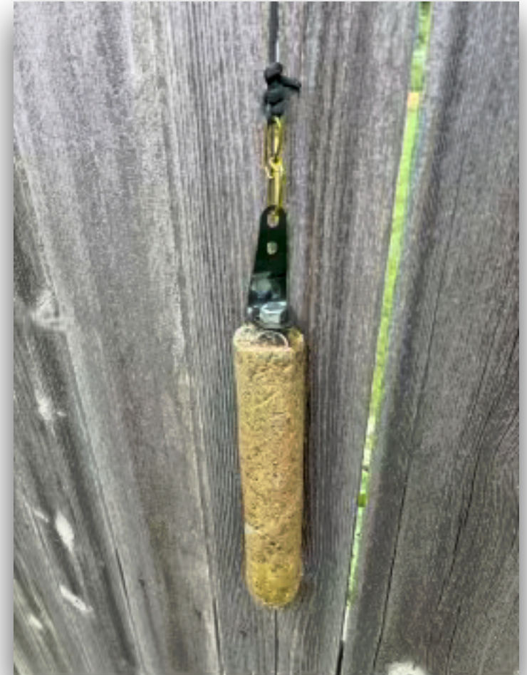
Counterweight, attached to end of para-cord (before attaching PVC pipe to fence)
