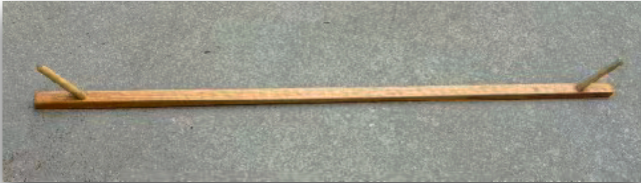
Empty "ParaKeeper" stick, on its back. (Maple dowels were glued into a 3-foot oak "1x1", then whole assembly was given two coats of thick, glossy polyurethane, for weather protection.)
