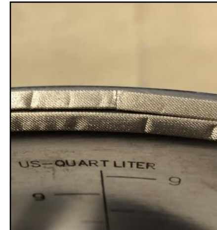
Rim/lip, showing where the strip's ends meet, to form a gap, in the outer-run of gasketing
