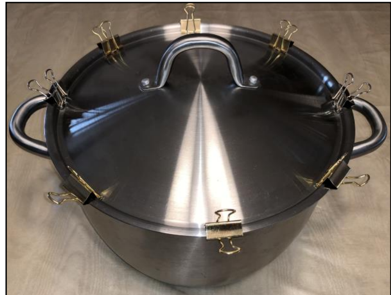
"Buttoned-up" Faraday Shield--a salvaged, stainless cooking pot!
