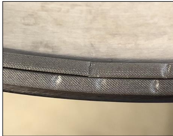
Rim/lip, showing gap in inner-run of gasketing, positioned "opposite" (i.e., on other side of can)
