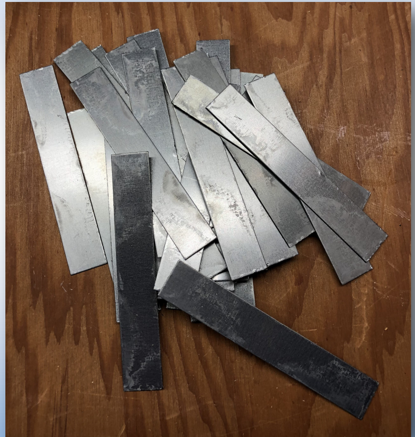
Try to get most of the rectangular E-core pieces out, first
