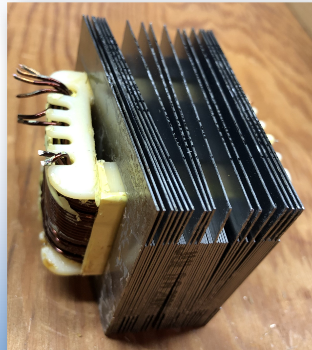
The laminations are almost falling out now.
