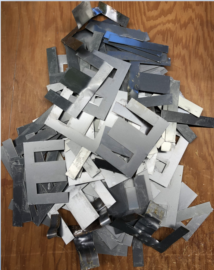
All of the iron core pieces, after removal
