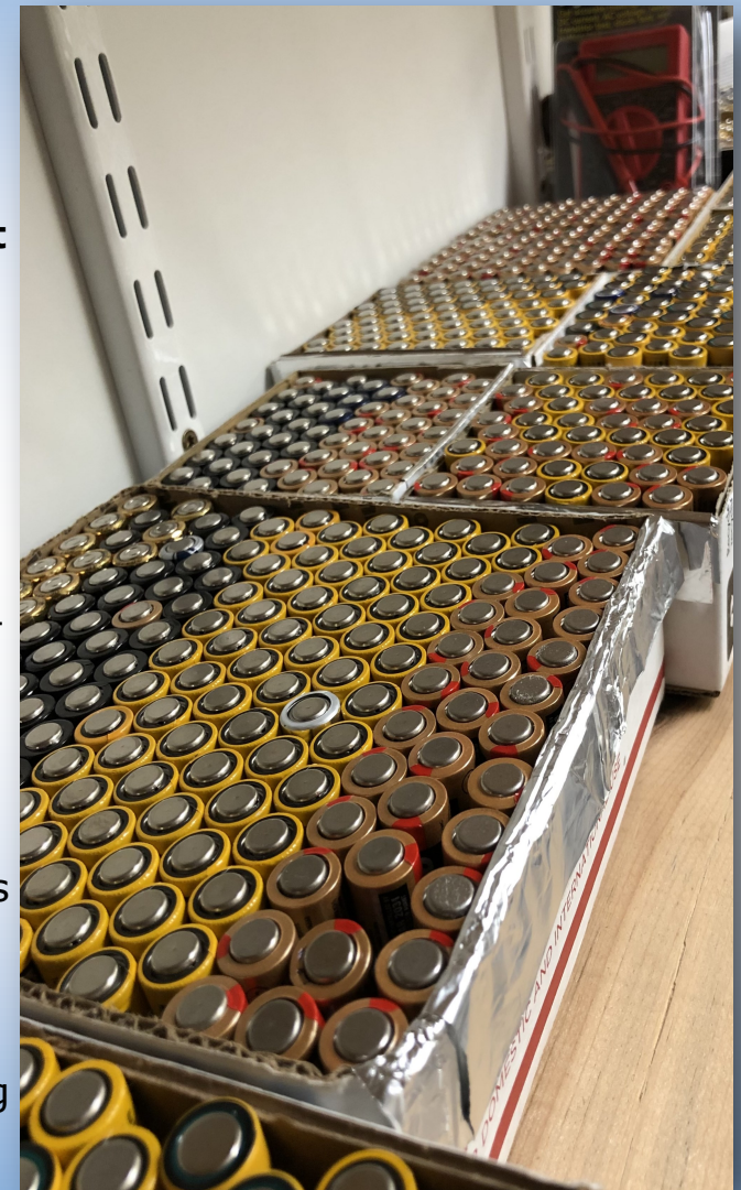
Storing used, alkaline, AA cells, "vent-end up."
