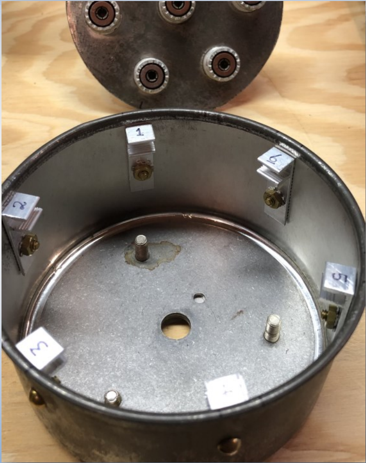
Brackets mounted on the inside of the can.
