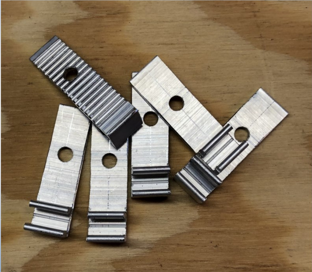
Drilled brackets (side holes).
