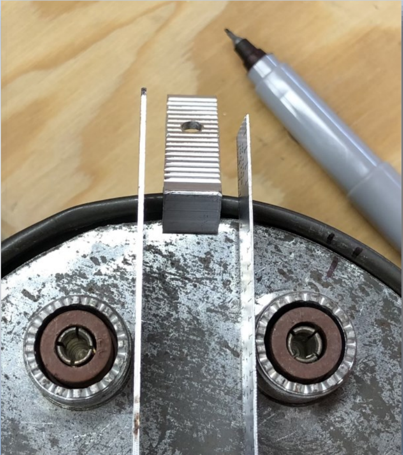
Marking the locations of the brackets on the can.
