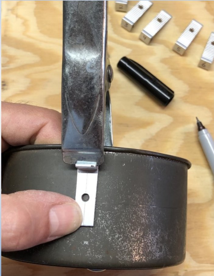
Marking each bracket's side-hole locations, on the outside of the can
