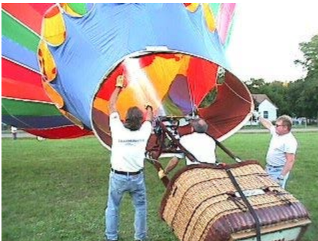
Doug WAØVEZ operating the burner to place hot air into the balloon envelope. The burner puts out a "couple" million BTUs of heat!!
